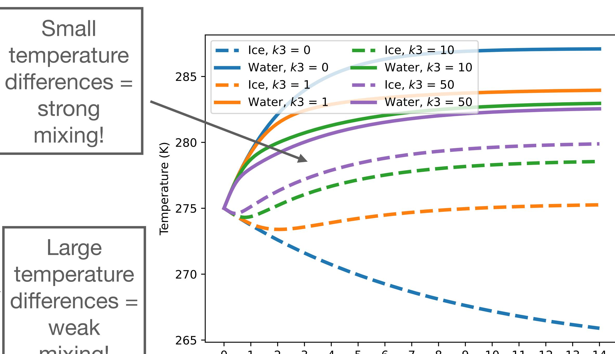
Results for **only linear heat transport**: not much mixing for small values of k!
